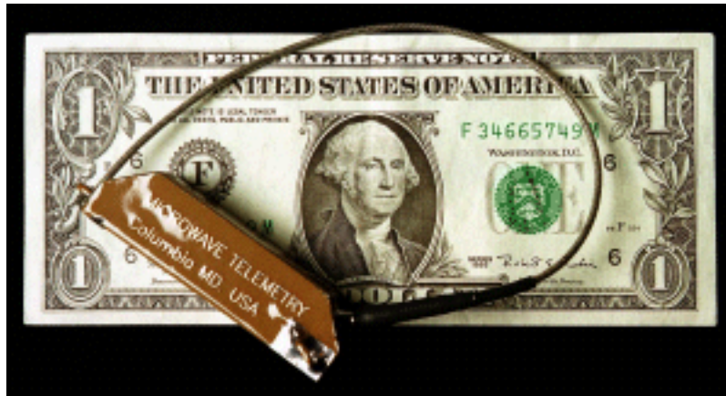
The transmitter that attaches to the wing of the Albatross is shorter than a dollar bill. Picture from http://www.wfu.edu/albatross
